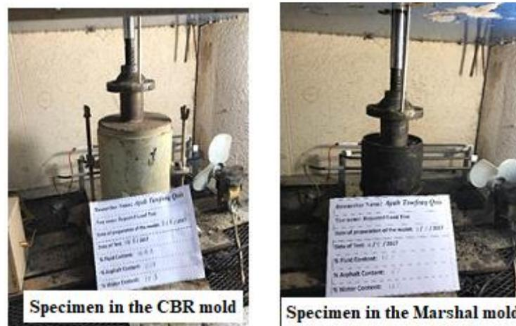
Figure 5. Both specimen sizes under test setup
