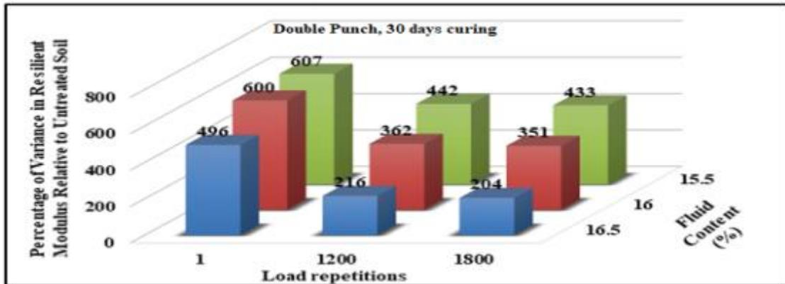
**Figure 7. Change in resilient modulus for several fluid content under double punch**
