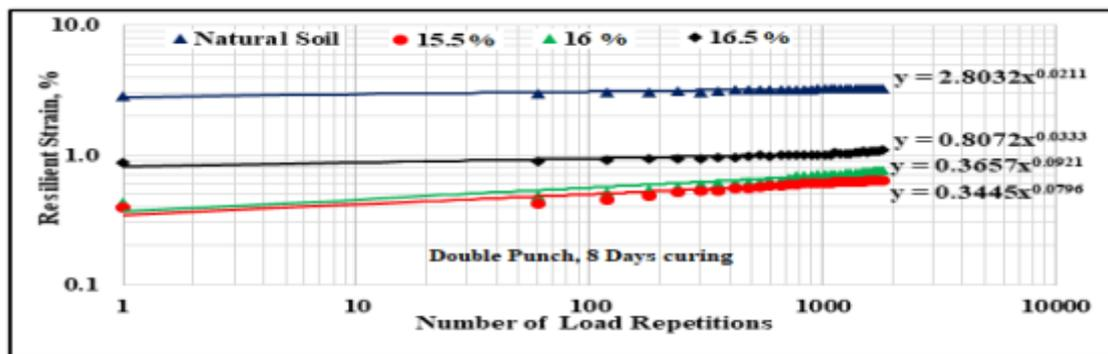
**Figure 8. Resilient strain versus number of load repetitions relation**
