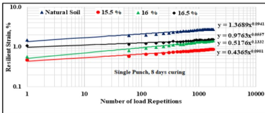
Figure 10. Resilient strain versus number of load repetitions for single punching shear
