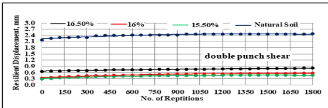
Figure 14. Variation of resilient displacement under double punch shear stress
