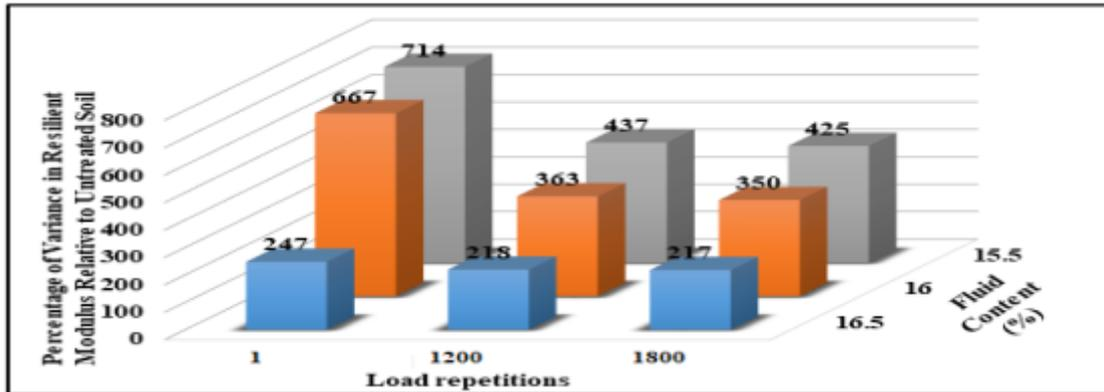
Figure 9. Change in resilient modulus for several fluid content under double punch
