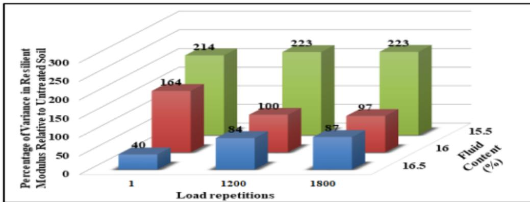
**Figure 11.** Change in resilient modulus for several fluid content under single punch
