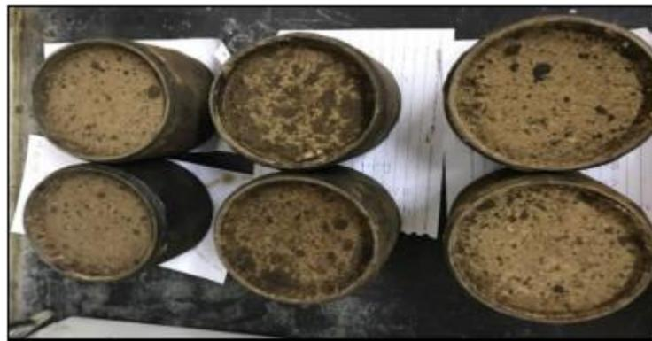
*Figure 3. Specimens for double punching shear repeated load test.*
