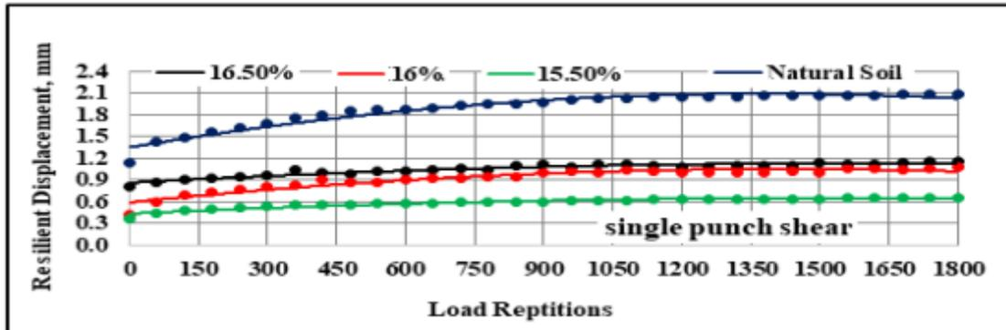
Figure 13. Variation of resilient displacement under single punch shear stress
