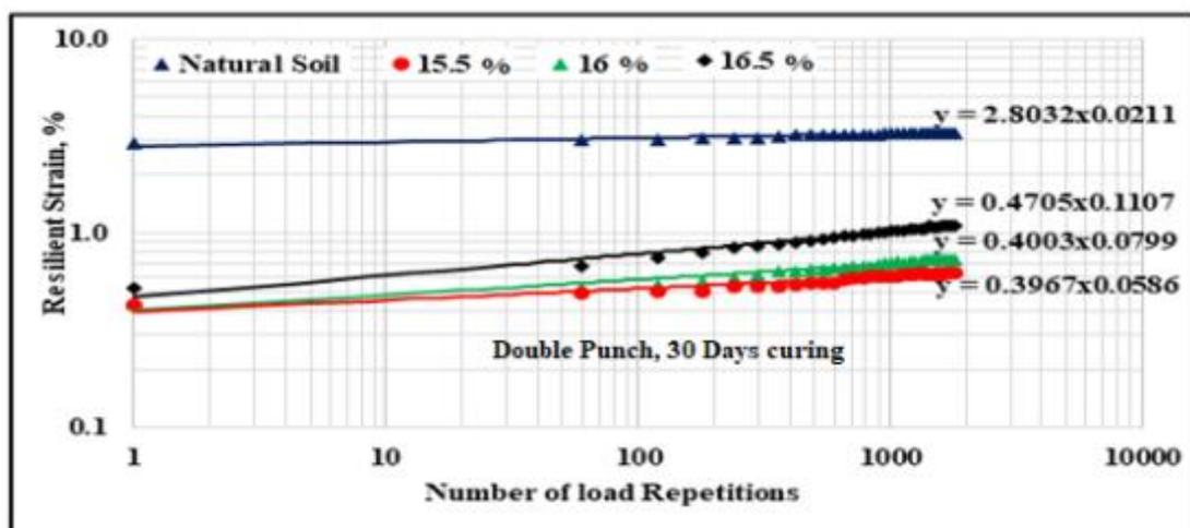
**Figure 6.** Resilient strain behavior for double punching shear test
