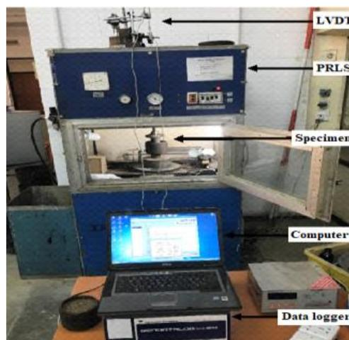
*Figure 4. Test setup using the PRLS*
