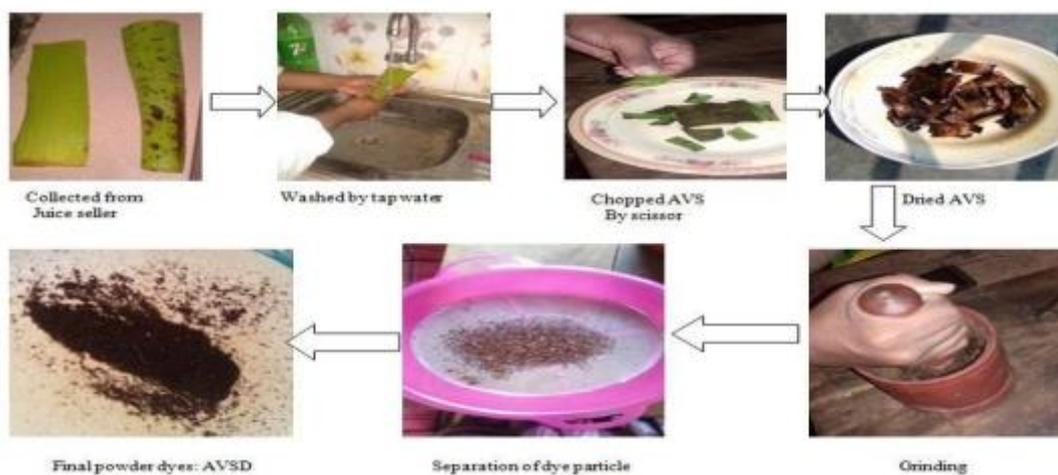
**Figure 1.** Procedure for the preparation of solid dyes (AVSD)
