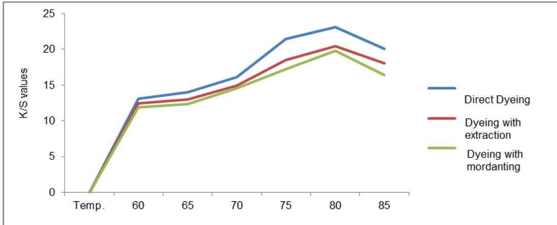
Figure 7. Effect of Temperature on colour strength (AVSD method)
