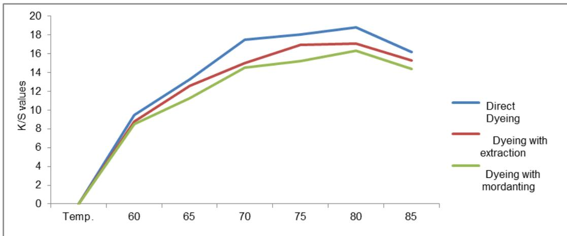
Figure 8. Effect of Temperature on colour strength (AVSS method)
