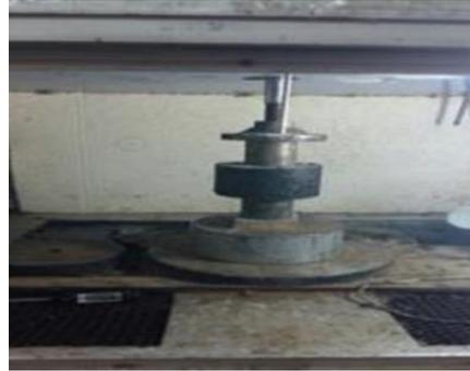
*Figure 3. Repeated double punching shear test*
