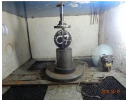
*Figure 2. Repeated indirect tensile strength test*
