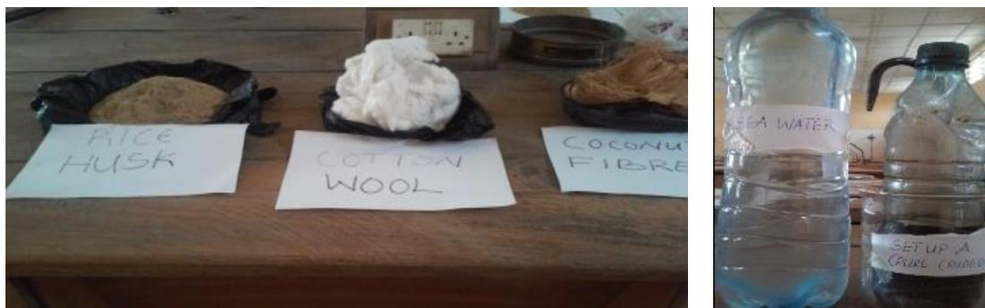
*Figure 1. Samples of Rice husk, Cotton wool, Coconut fibre, Sea water and Crude Oil used*
