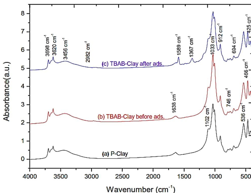
**Figure 3.** FTIR spectra of P-Clay and TBAB-Clay samples
