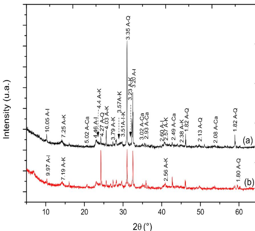
**Figure 2.** XRD patterns of P-Clay (a) and TBAB-Clay (b) (I: Illite, K: Kaolinite, Ca: Calcite, Q: Quartz)
