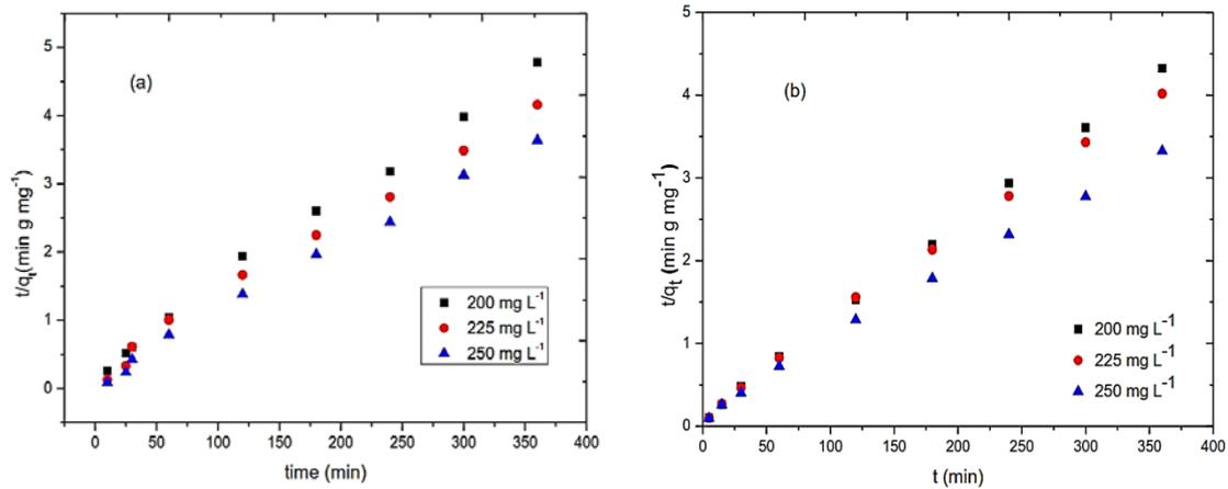
**Figure 7.** Pseudo-second-order kinetic modelling of CV adsorption on P-Clay (a) and TBAB-Clay (b). Conditions: CV concentration (■) 200, (●) 225 and (▲) 250  $\text{mg L}^{-1}$ , 50.0 mL, 0.10 g, 7.3 pH, 28°C, 500 rpm
