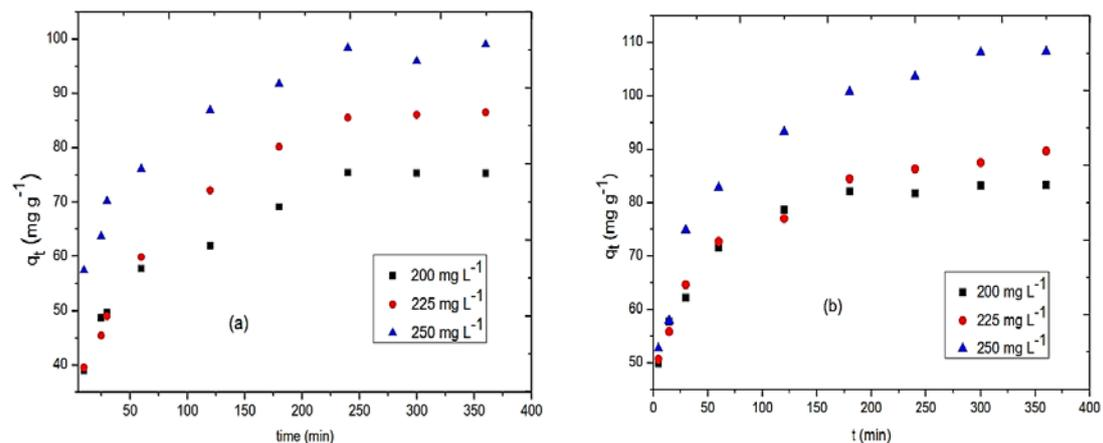
**Figure 6.** Effect of contact time and initial concentration of CV adsorption on P-Clay (a) and on TBAB-Clay (b). Conditions: CV concentration (■) 200, (●) 225 and (▲) 250  $\text{mg L}^{-1}$ , 50.0 mL, 0.10 g, 7.3 pH, 28°C, 500 rpm
