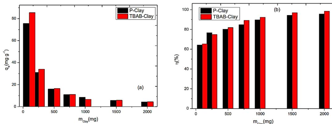
Figure 5. The effect of P-Clay and TBAB-Clay quantity on CV adsorption over the (a) adsorption capacity and (b) removal efficiency; Conditions: 50.0 mL,  $200 \text{ mg L}^{-1}$ , 7.3 pH,  $28^\circ\text{C}$ , 500 rpm
