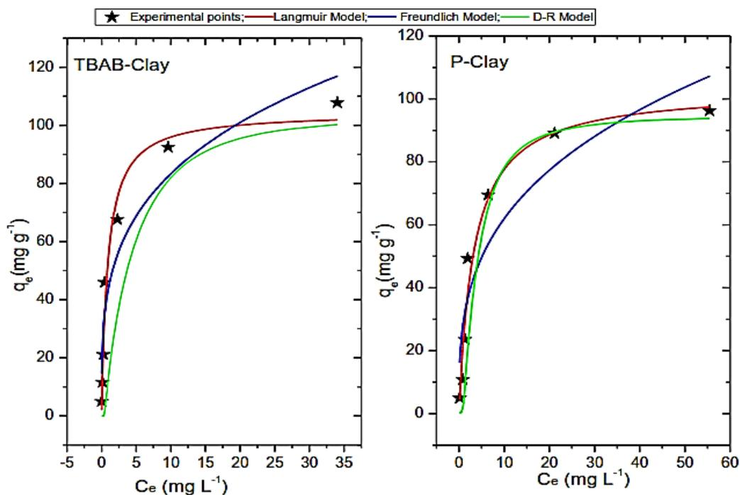
**Figure 8.** Non-linear isotherm modelling of CV adsorption on P-Clay and TBAB-Clay
