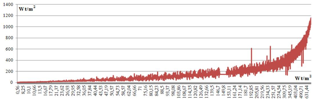
**Figure 6.** Dependence of solar radiation on the surface of the panel from solar radiation on the surface of the earth (during March-April-May).
