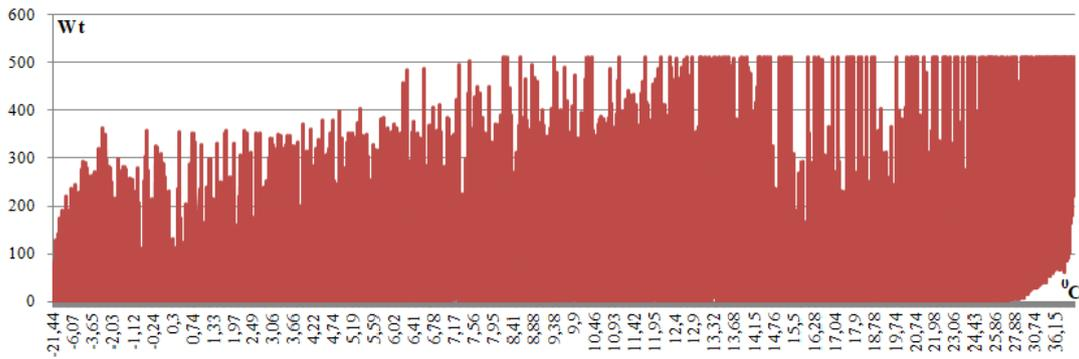
**Figure 3.** Dependence of active power on panel temperature (during the year).
