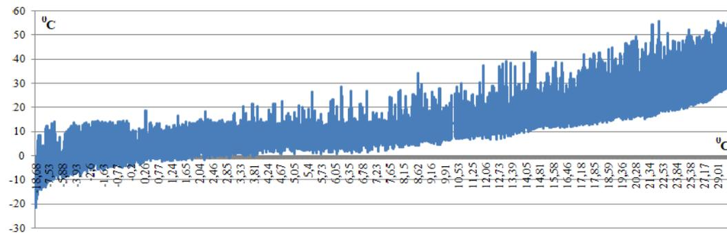
**Figure 5.** Panel temperature dependence on ambient temperature (during the year).
