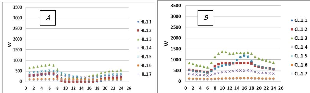
Figure 4. Thermal insulation heating and cooling loads, where: (A) is heating load, (B) is cooling load.
