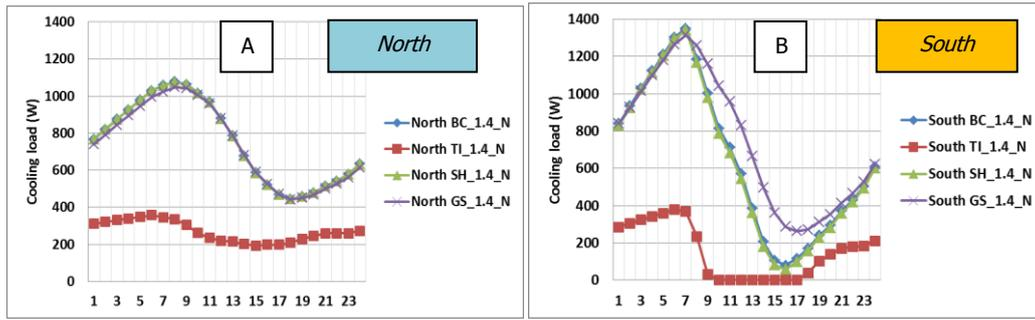
**Figure 7.** Cooling load North and South zones with respect to all suggested designs, where: (A) is North facing, (B) is South facing zones.
