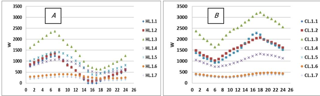
Figure 3. Base case heating and cooling load, where: (A) is heating load, (B) is cooling load.
