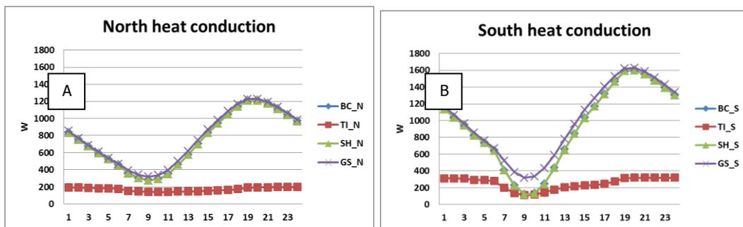
**Figure 8.** Heat conduction in North (A) and South (B) zones with respect to all suggested designs.
