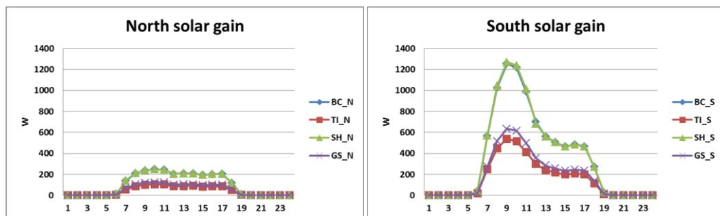
**Figure 9.** Solar heat gain in North and South zones with respect to all suggested designs.
