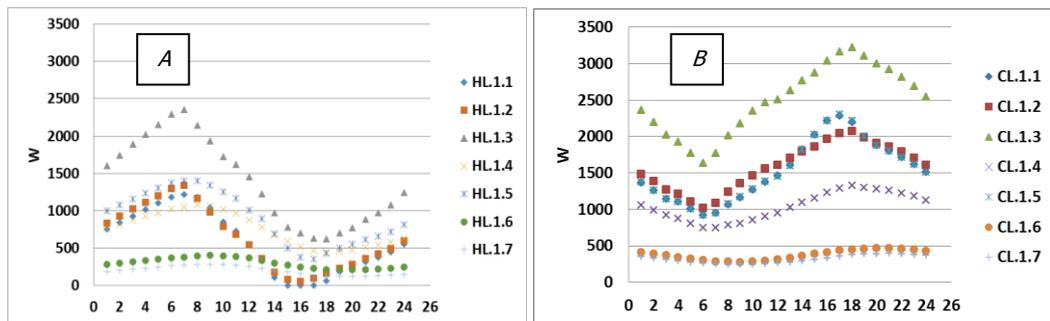
Figure 5. Shading devices heating and cooling loads, where: (A) is heating load, (B) is cooling load.
