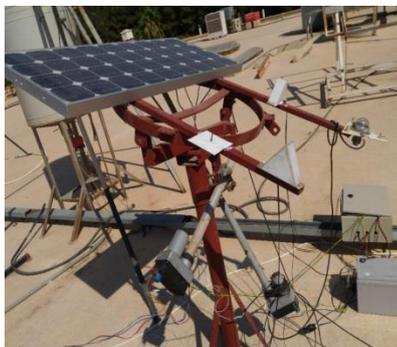
**Figure 1.** Dual and single axis sun tracker.
