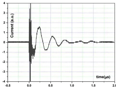
**Figure 3.** Discharge current signal from IEC plasma.
