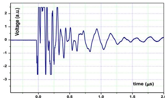
**Figure 4.** Discharge voltage signal from IEC plasma.
