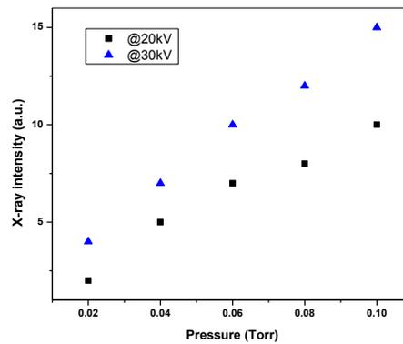
**Figure 11.** X-ray production as a function of pressure for different voltages [13].
