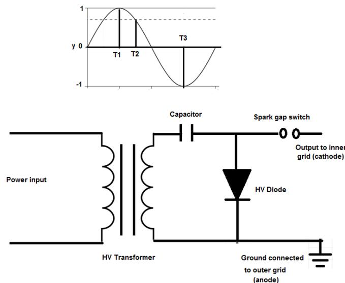
**Figure 2.** Circuit diagram of the power supply.
