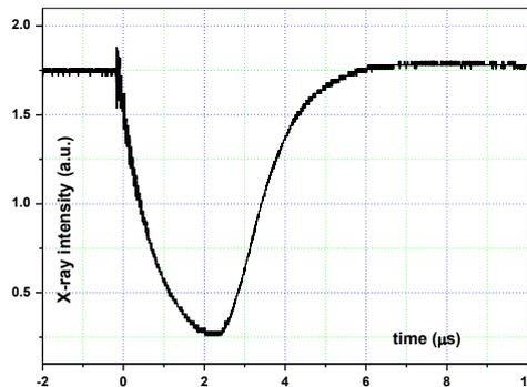
**Figure 9.** Signal of scintillation hard X-ray detector for nitrogen plasma.
