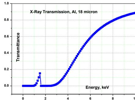
**Figure 6.** Graph showing the X-ray transmission of 18m thick sheet of Al, Z=13.
