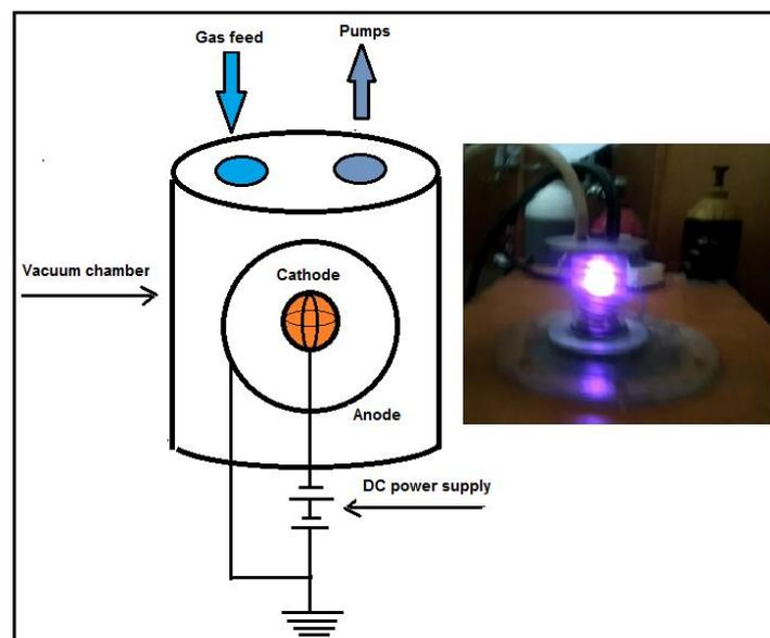
**Figure 1.** Schematic diagram and photo of experimental setup.
