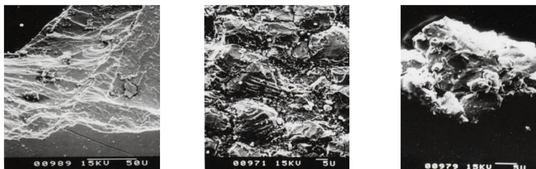
(a) quasi-cleavage (b) Granular mode with torn edges (c) Granular mode with torn edges
