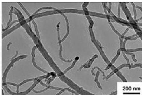
*Figure 1. TEM image of CNTs prepared by CCVD.*
