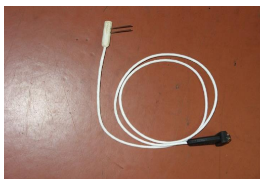
Figure 20. Dual-needle sensors for volumetric specific heat capacity and diffusivity measurements (30 mm).
