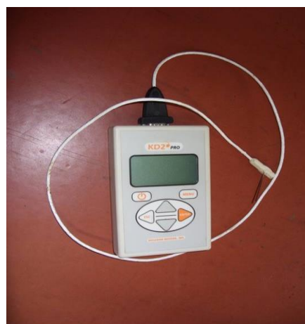
Figure 18. Single-needle sensors for thermal conductivity and resistivity measurements (6 cm) for liquids.
