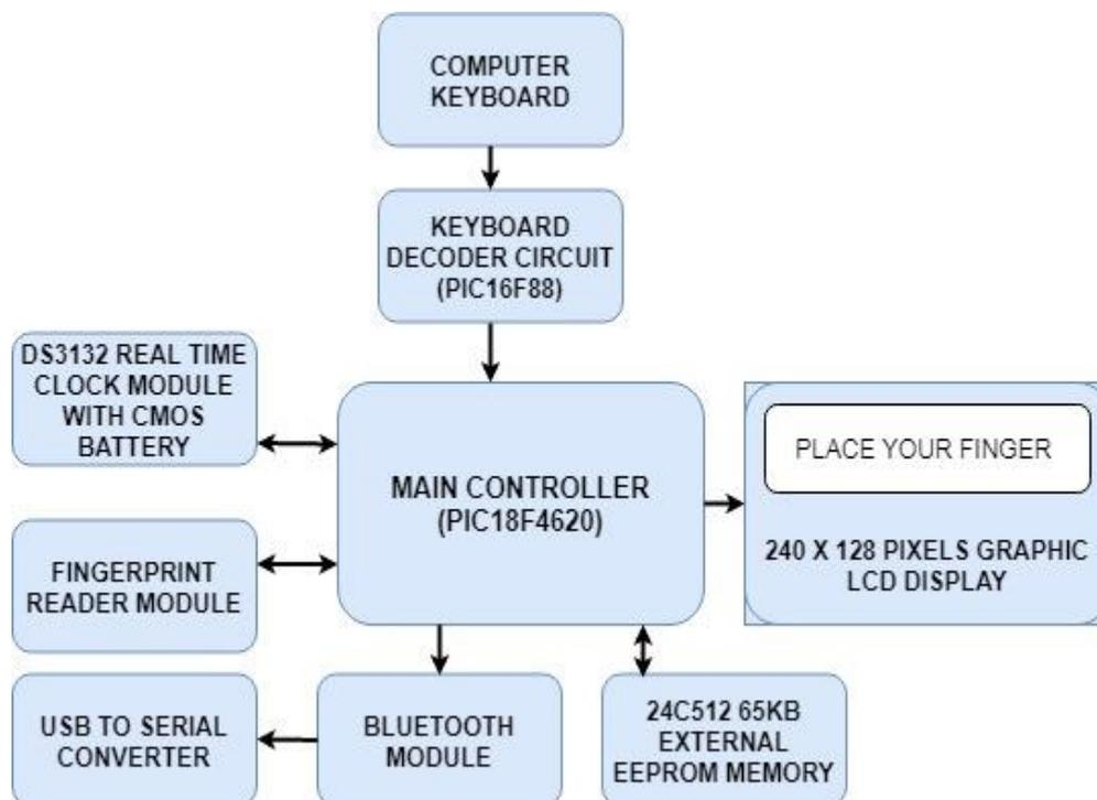
Figure 1. Main Board Block Diagram of the System.
