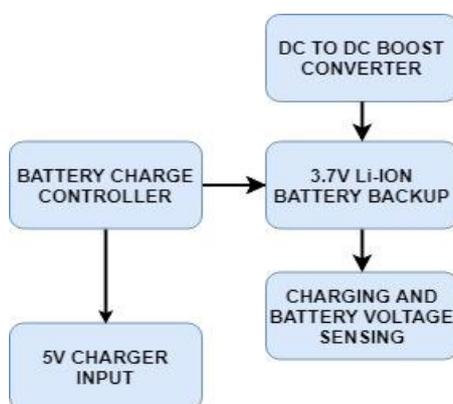
Figure 2. Block Diagram of Power Section.
