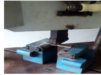
Figure 8. Flexural Test Set-up.
