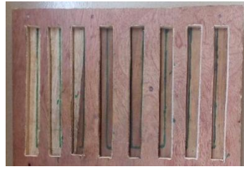
Figure 7. Flexural Specimen mold.
