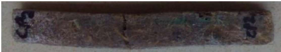
Figure 9. Deformed Flexural Test Specimen.
