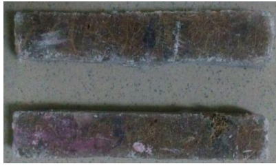
Figure 6. Flexural Test Specimens.
