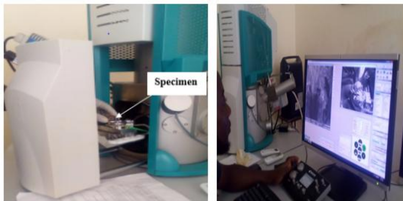
Figure 5. Tescan VEGA3 Scanning Electron Microscope set-up and its usage.
