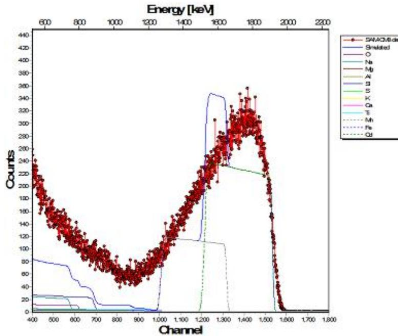
*Figure 12. Elemental Composition of Sample Deposited in 4 minutes obtained using RBS Techniques.*
