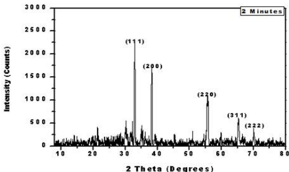
**Figure 7.** X–Ray Diffraction pattern of CdMnO<sub>2</sub> Thin film deposited at 2 minutes.
