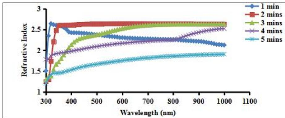
Figure 5. Plot of refractive index versus wavelength (nm) of CdMnO<sub>2</sub> thin films at various time of deposition.
