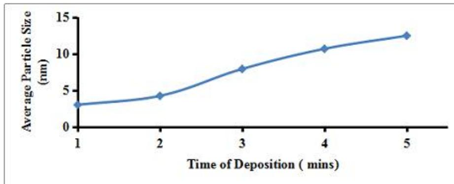
**Figure 10.** Plot of Average Particle Sizes of Deposited Films against Deposition Time.
