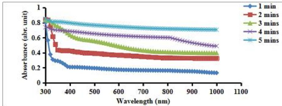
**Figure 2.** Plot of absorbance (abr. unit) versus wavelength (nm) of CdMnO<sub>2</sub> Thin films at various time of deposition.
