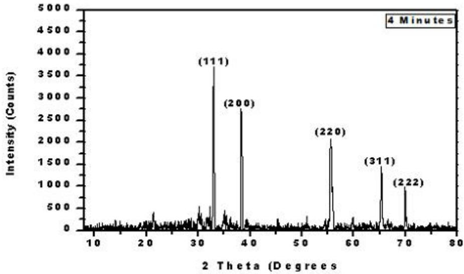
**Figure 8.** X– Ray Diffraction pattern of CdMnO<sub>2</sub> Thin film deposited at 4 minutes.
