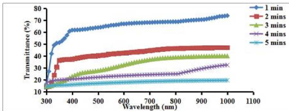
**Figure 3.** Plot of transmittance versus wavelength (nm) of CdMnO<sub>2</sub>Thin films at various time of deposition.
