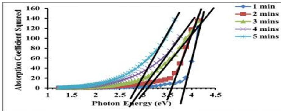
Figure 6. Plot of absorption coefficient squared versus wavelength (nm) of CdMnO<sub>2</sub> thin films at various time of deposition.
