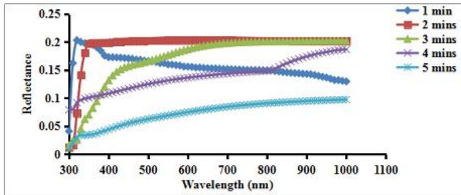
Figure 4. Plot of reflectance versus wavelength (nm) of CdMnO<sub>2</sub> thin films at various time of deposition.
