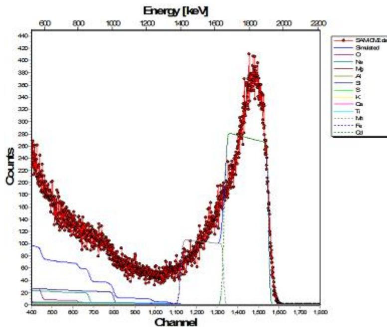
**Figure 11.** Elemental Composition of Sample Deposited in 2 minutes obtained using RBS Techniques.
