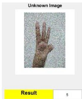
**Figure 7.** Testing Result for Number '3' with Speckle Noise with Variance 0.04.
