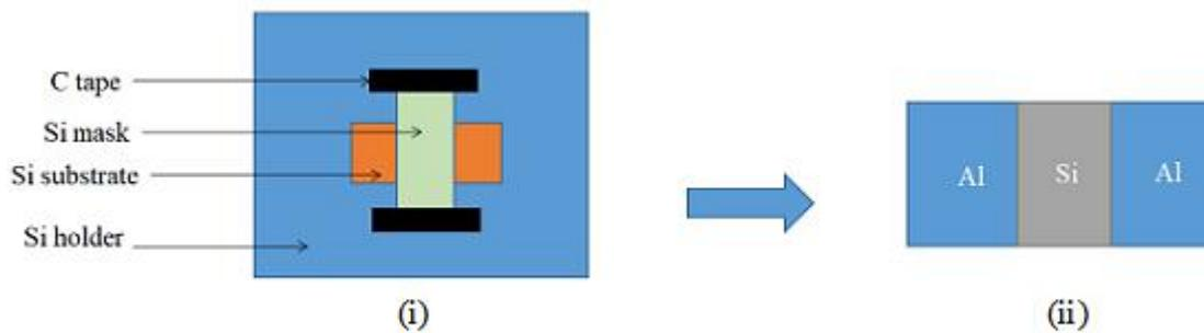
**Figure 2.** (i) Specimen Setup before Deposition, (ii) Desired Result Specimen after Deposition.
