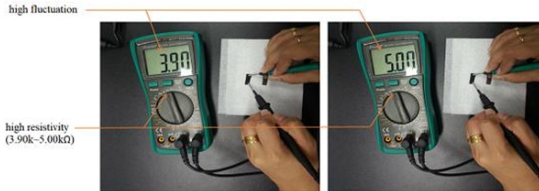
**Figure 7.** Test of Specimen Treated without HF Acid.
