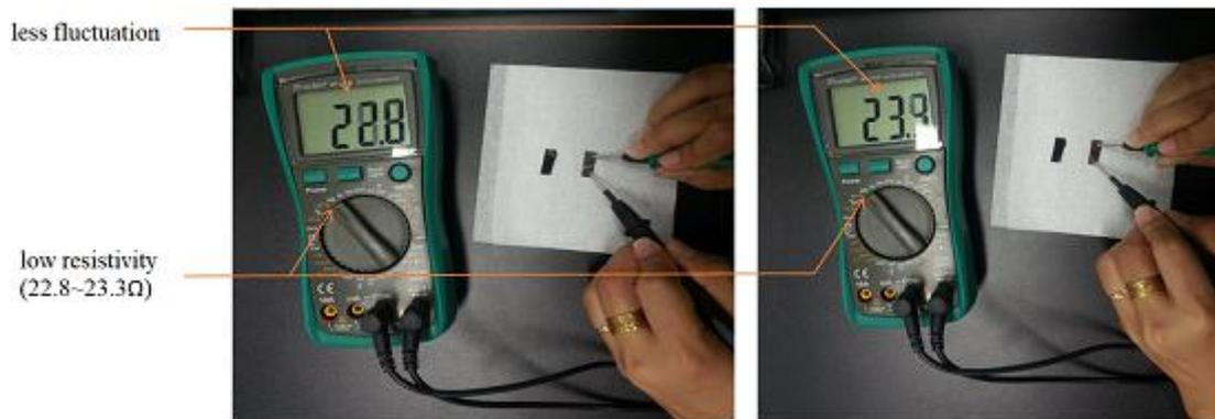
**Figure 8.** Test of Specimen Treated with HF Acid.
