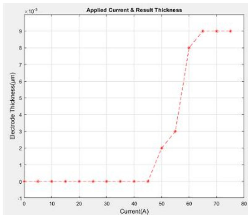
**Figure 9.** Condition of Thickness of Electrode due to Applied Current.
