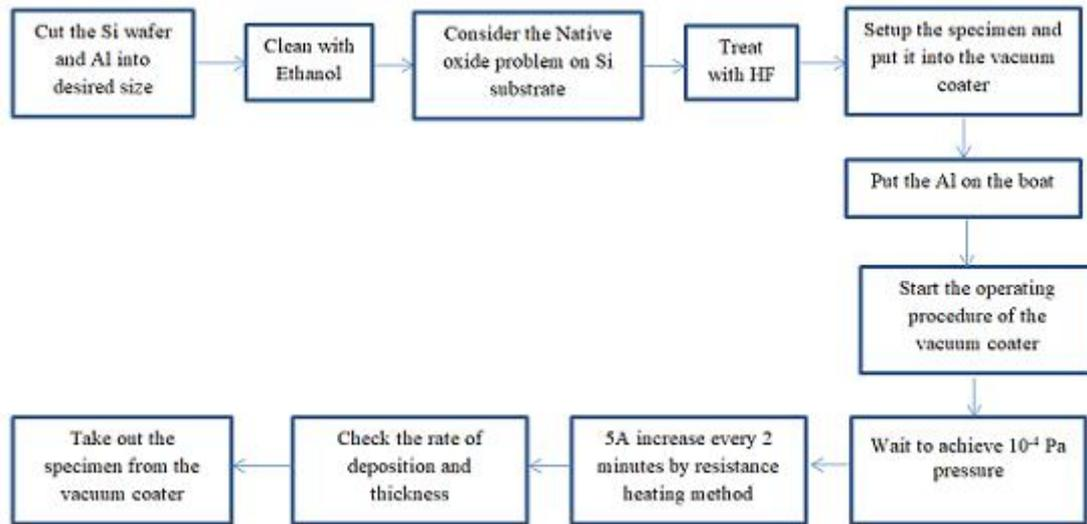
**Figure 1.** Block Diagram of Fabrication Procedure.
