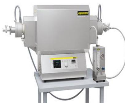
**Figure 4.** A photograph of the tube furnace used for steam activation of coke.
