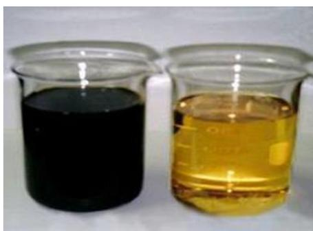
**Figure 3.** Image of used and fresh oil sample.
