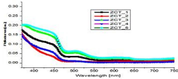
**Figure 4.** Plot of Reflectance against Wavelength (nm) for ZCT<sub>1</sub>, ZCT<sub>2</sub>, ZCT<sub>3</sub>, ZCT<sub>4</sub> and ZCT<sub>5</sub> thin films.
