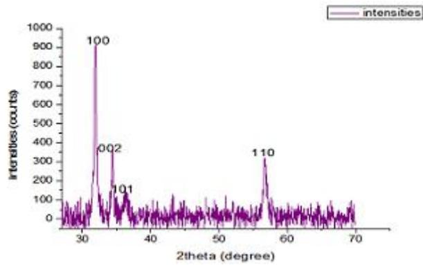
**Figure 10.** Plot of intensities versus 2 theta for sample ZCT<sub>4</sub>.
