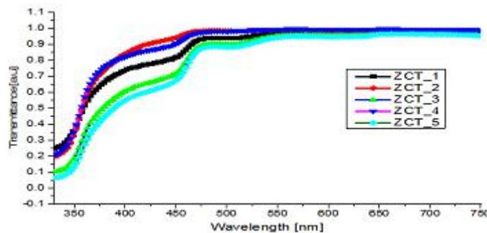
**Figure 3.** Plot of Transmittance against Wavelength for Samples ZCT<sub>1</sub>, ZCT<sub>2</sub>, ZCT<sub>3</sub>, ZCT<sub>4</sub> and ZCT<sub>5</sub>.
