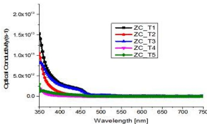
**Figure 8.** Graph of Optical Conductivity against Wavelength (nm).
