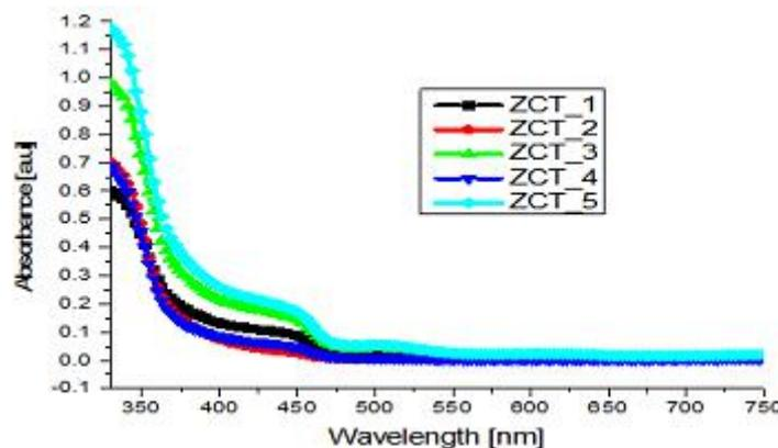
**Figure 2.** Plot of Absorbance against Wavelength for ZCT<sub>1</sub>, ZCT<sub>2</sub>, ZCT<sub>3</sub>, ZCT<sub>4</sub> and ZCT<sub>5</sub>.
