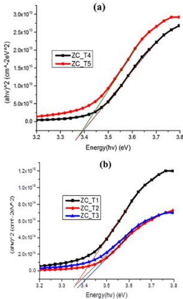
**Figure 9.** (a): plot of  $(ahv)^2$  against  $(hv)$  for samples ZCT<sub>1</sub>, ZCT<sub>2</sub> and ZCT<sub>3</sub> (b): Plot of  $(ahv)^2$  Vs  $(hv)$  for samples ZCT<sub>4</sub> and ZCT<sub>5</sub>.
