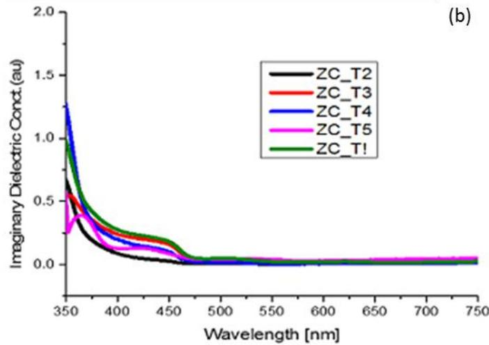
**Figure 7.** (a) Plot of Real Dielectric Constant against Wavelength (nm), (b) Plot of Imaginary Dielectric Constant against Wavelength for Samples ZCT<sub>1</sub>, ZCT<sub>2</sub>, ZCT<sub>3</sub>, ZCT<sub>4</sub> and ZCT<sub>5</sub>.
