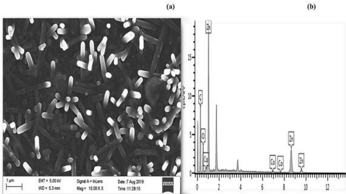
**Figure 11.** (a) SEM image of sample ZCT<sub>4</sub>. (b) Energy Dispersive X-ray Spectroscopic Spectra of ZCT.
