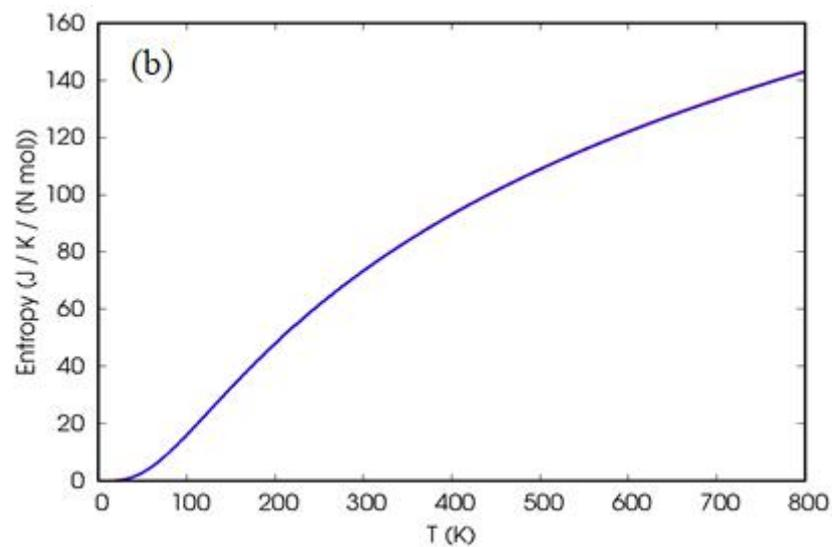
**Figure 4b.** Entropy of RhVSi hH alloy with temperature change.
