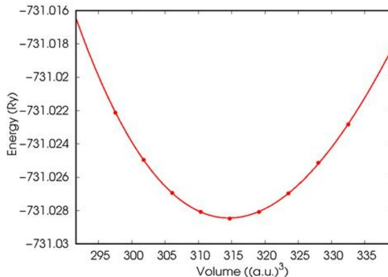
**Figure 2.** Lattice optimization for the minimum energy versus volume as fitted to the Murnaghan equation of state.
