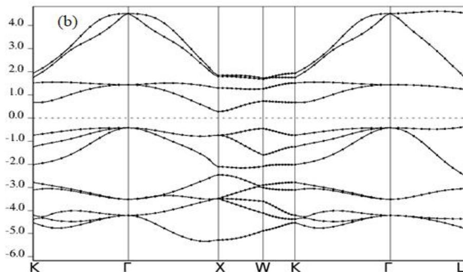
**Figure 3b.** Band-structure calculation of RhVSi half Heusler alloy using the DFT-GGA approximation.
