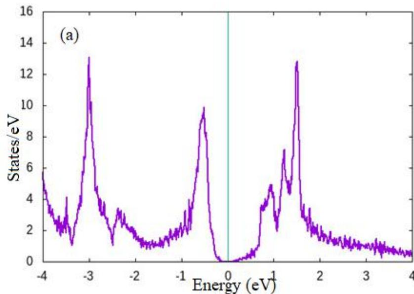
**Figure 3 a.** Total electronic density of states of RhVSi half Heusler alloy using the DFT-GGA approximation.
