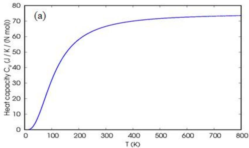
**Figure 4a.** Specific heat capacity  $C_v$  of RhVSi hH alloy.
