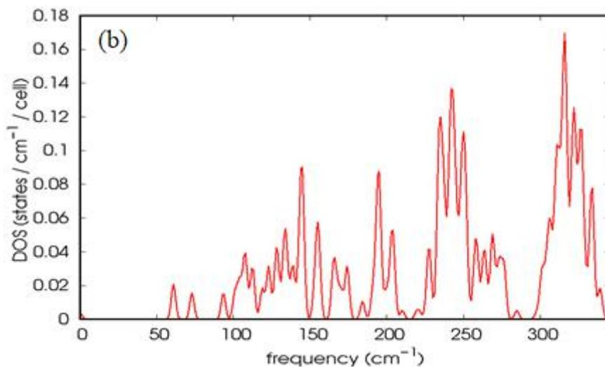
**Figure 5b.** Density of states frequency of RhVSi hH alloy.
