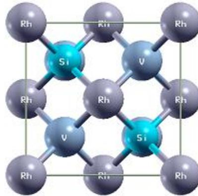
**Figure 1.** The most stable crystal structure of RhVSi at the atomic positions (0, 0, 0), (0.25, 0.25, 0.25) and (0.75, 0.75, 0.75) for Rh, V, Si respectively.
