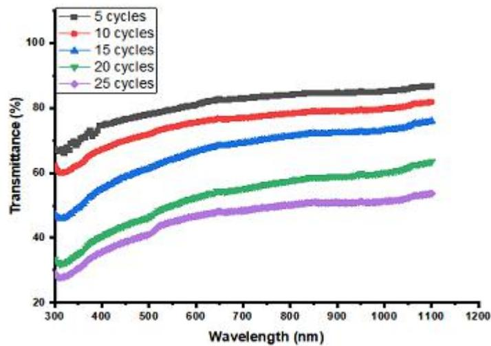
*Figure 5. Graph of transmittance plotted against wavelength for lead iodide thin films deposited at different SILAR cycles.*
