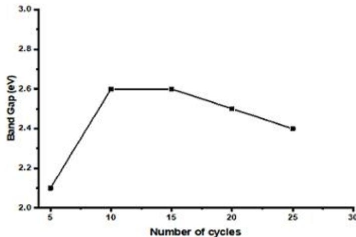
**Figure 8.** Graph of energy band gap plotted against number of SILAR cycles.
