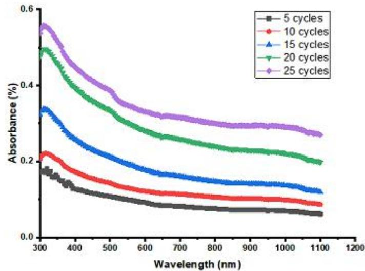
*Figure 4. Graph of absorbance plotted against wavelength for lead iodide thin films deposited at different SILAR cycles.*
