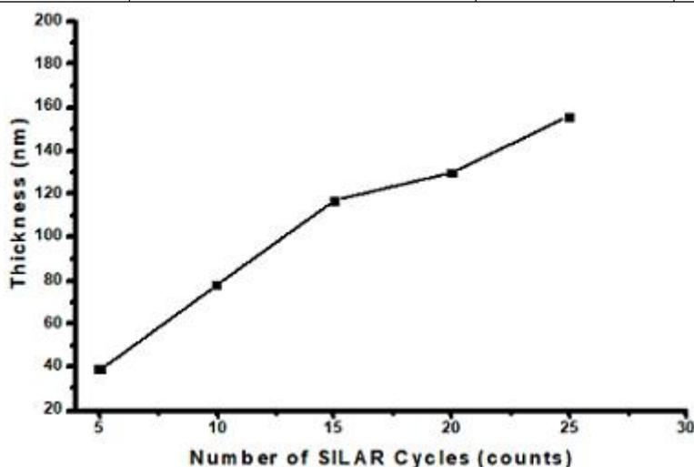
**Figure 2.** Graph of thickness plotted against number of SILAR cycles.
