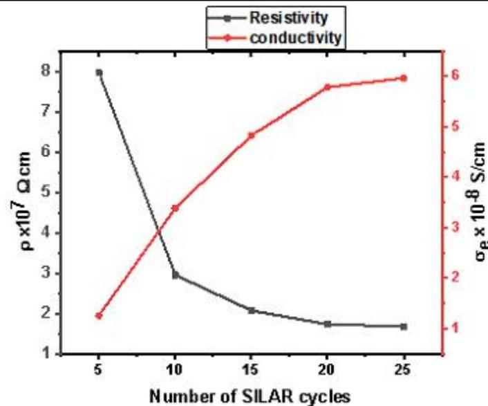
**Figure 3.** Variation of electrical properties of Lead iodide thin films with number of SILAR cycles.
