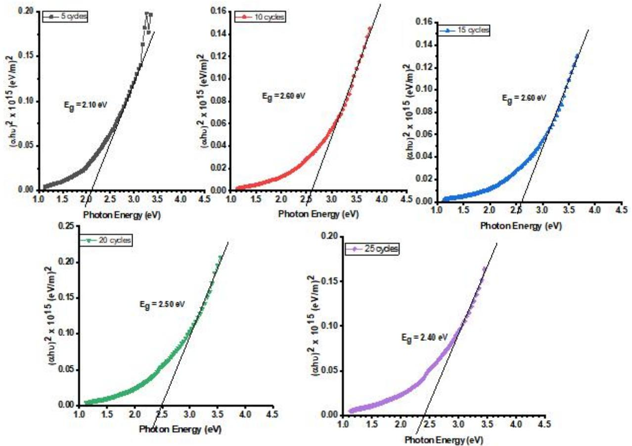
**Figure 7.** Graph of  $(\alpha h\nu)^2$  plotted against photon energy (eV) for lead iodide thin films deposited at different SILAR cycles.
