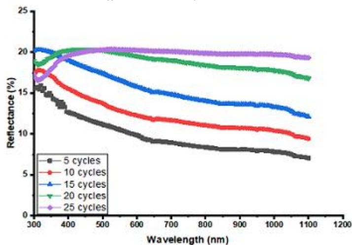
*Figure 6. Graph of reflectance plotted against wavelength for lead iodide thin films deposited at different SILAR cycles.*
