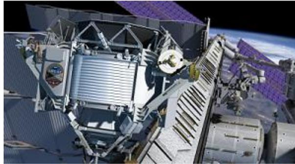
*Figure 3. AMS-02 detector at the International Space Station (ISS).*
