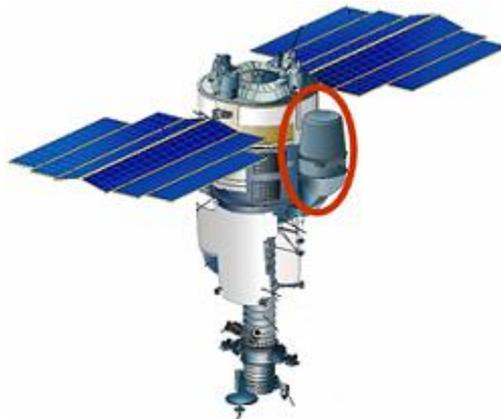
*Figure 1. “PAMELA” in a container on the Resurs-DK satellite.*
