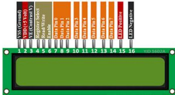
Figure 3. Pictorial Diagram of a 16 ×2 LCD.
