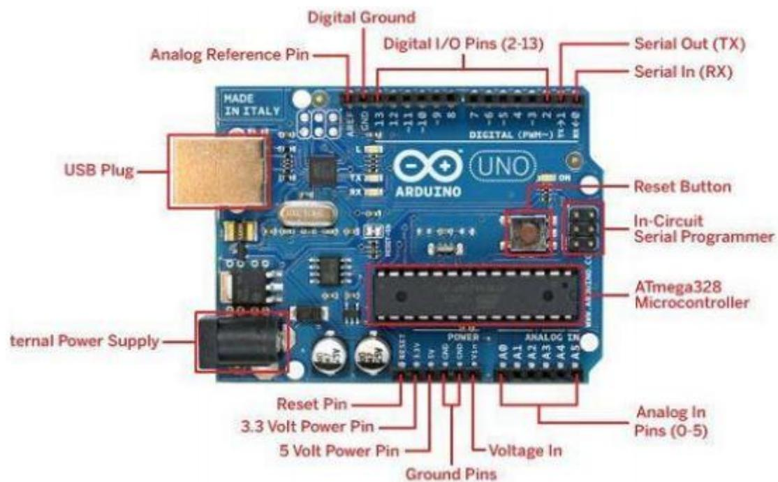
*Figure 1. Pictorial Description of an Arduino Uno Board [13]*
