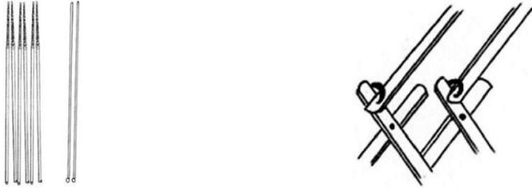
**Figure 8.** Ejector rob. **Figure 9.** The connection between ejector rod and enclosure bulkhead.
