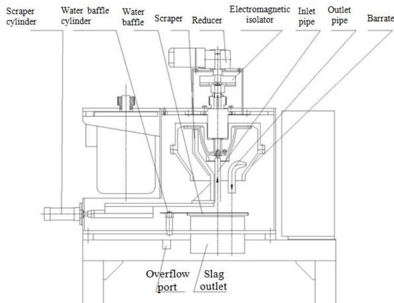
Figure 3. Centrifuge structure drawing.
