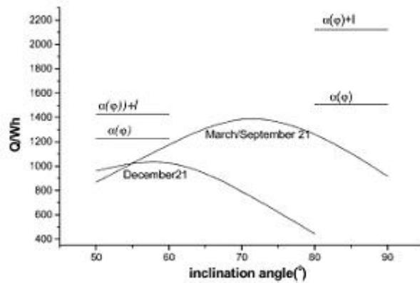
**Figure 11.** Dependence of the daily energy gain in different types of greenhouses. Different types illustrate the effects of the inclination angle of the wall at the shortest winter day and at equinox. The horizontal lines show the effects of different inclination angles without and with louvers.
