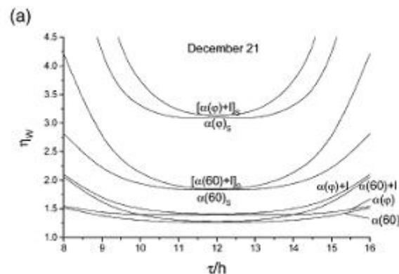
**Figure 10.** Dependence of the irradiance enhancement coefficient on time, the shortest day of the year and equinox at  $44^\circ$  NL in a greenhouse with reflecting walls inclined at optimum angles  $\alpha(60)$  and  $\alpha(70)$ , and with reflecting walls with variable inclinations.
