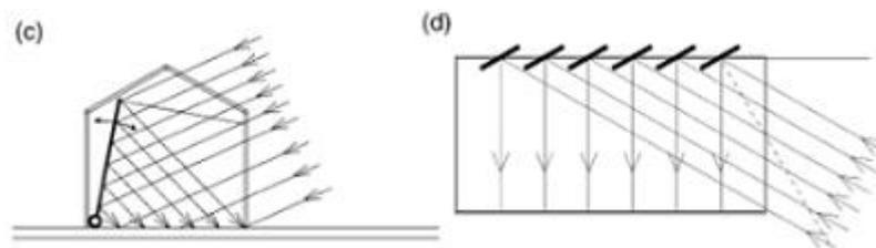
**Figure 2.** Greenhouse types according to the applied mode of reflection of solar radiation: (a) fixed vertical reflecting wall (b) fixed inclined reflecting wall (c) reflecting wall with variable inclination (d) reflecting wall with louvers.
