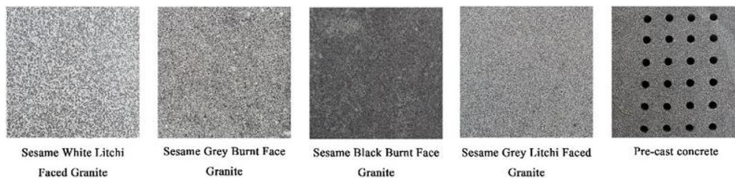
**Figure 9.** Paving materials for roof gardens
