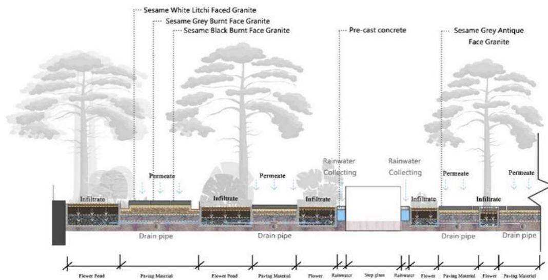
**Figure 11.** Microclimate elevation analysis of roof garden paving materials.
