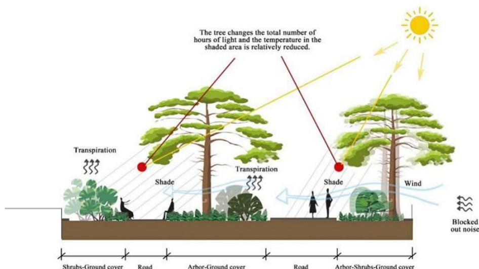
**Figure 8.** Roof garden plant microclimate elevation analysis.
