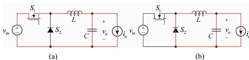
Figure 2. Two switching states (with continuous inductor current) (a)  $S_1$  ON, (b)  $S_2$  ON.
