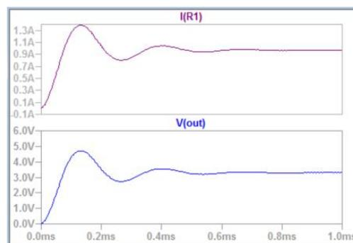
**Figure 8.** Output Voltage and Current of the DC to DC Buck Converter.
