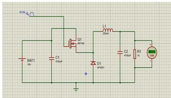
*Figure 4. Buck Converter with 16V Input.*
