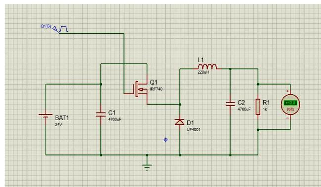
*Figure 5. Buck Converter with 24V Input.*
