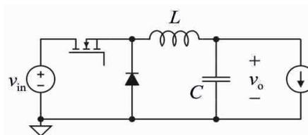
Figure 1. DC to DC Buck Converter.
