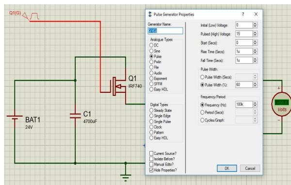
**Figure 7.** Checking Duty Cycle.
