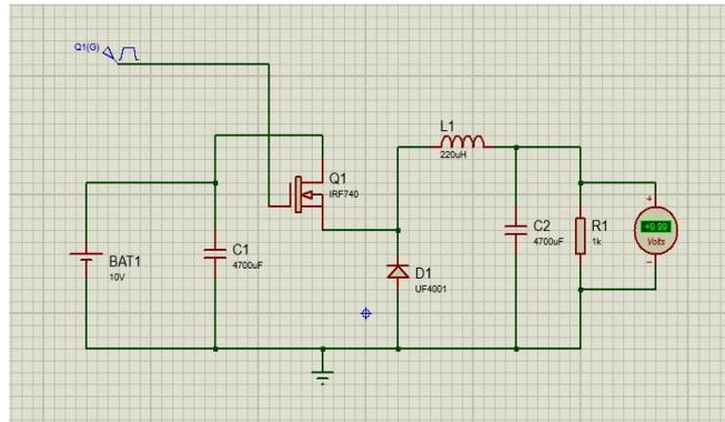
**Figure 6.** Buck Converter with 10V Input.
