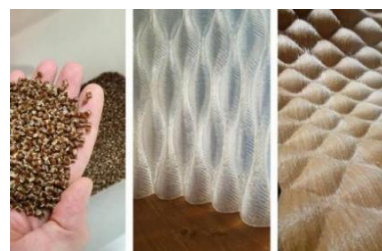
Figure 3. From left to right: polylactic acid pellets, upright model, model surface.
