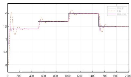
Figure 9. EC value simulation curve.
