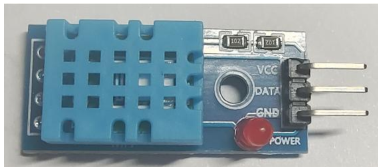
Figure 2. DHT11 temperature and humidity sensor.
