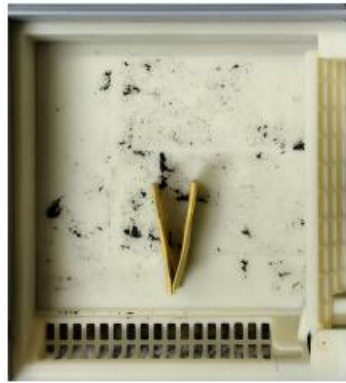
Figure 6. V-shaped splitter cone in the intake chamber.
