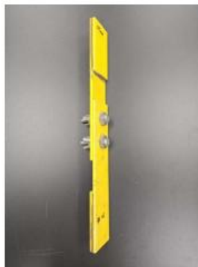
Figure 2. One-sided bolted GFRP joint.
